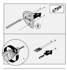
8) Remove cover of hand shower cradle (N). Install cradle and mounting plate (O). Secure with three screws (M). Replace cover on hand shower cradle.
