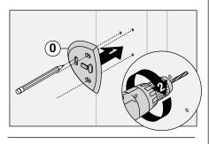
**Option:** Place mounting plate (O) in position, mark and drill 3/16" holes into wall. Install anchors.
