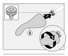
6) Install wall elbow (B) to pipe fitting. Turn clockwise to tighten.
