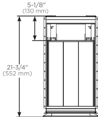
Top view for plumbing and sink clearance
