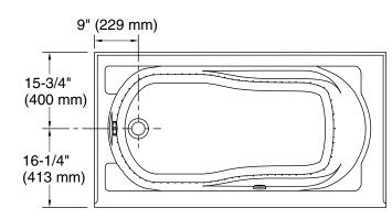
No change in measurements if connected with drain illustrated. (K-7213)
