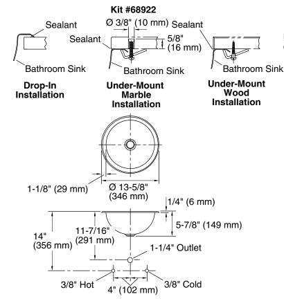
**Note:** Waterproof unprotected overhang area of the underside of wood counter.
