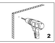
Drill 3/16" holes, make sure to keep drill level
