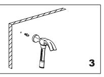
Insert plugs into drilled holes, using a hammer to tap the plugs in, be careful not to break tile
