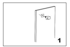
Install the hook (bolt) through the glass hole, make sure the rubber gaskets are between knob&glass.
