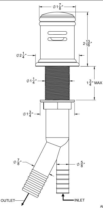
THROUGH-HOLE SPECIFICATIONS **RECOMENDED** <u>MAX</u> Ø 1-1/4" Ø 1-3/8" Ø 1-9/16"
