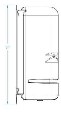
FEATURES Dimensional Tolerance ± 3/8". Dimensions needed for site preparation should be measured from the unit. Aquatic assumes no responsibility for preparatory work.
